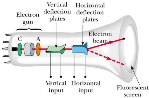
**Figure 23.26** Schematic diagram of a cathode ray tube. Electrons leaving the hot cathode C are accelerated to the anode A. In addition to accelerating electrons, the electron gun is also used to focus the beam of electrons, and the plates deflect the beam.
