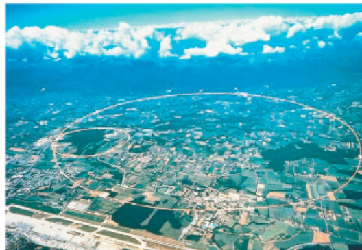
FIGURE 32-5 The large circle represents the position of the tunnel, about 100 m below the ground at CERN (near Geneva) on the French-Swiss border, which will house the LHC. The smaller circle shows the position of the Super Proton Synchrotron that will be used for accelerating protons prior to injection into the LHC.
