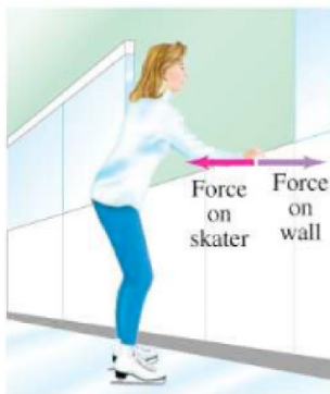
FIGURE 4-9 An example of Newton's third law: when an ice skater pushes against the wall, the wall pushes back and this force causes her to accelerate away.
