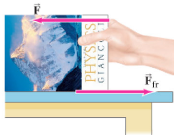
FIGURE 4–3 \vec{F} represents the force applied by the person and \vec{F}_{fr} represents the force of friction.
