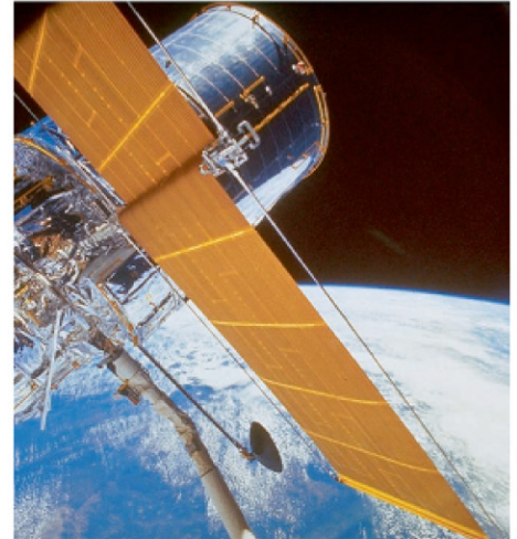
FIGURE 25–31 Hubble Space Telescope, with Earth in the background. The flat orange panels are solar cells that collect energy from the Sun.
