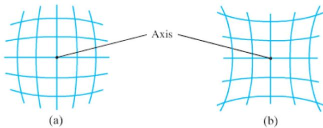
**FIGURE 25-25** Distortion: lenses may image a square grid of perpendicular lines to produce (a) barrel distortion or (b) pincushion distortion. These distortions can be seen in the photograph of Fig. 23-29d.
