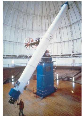
FIGURE 25–20 This large refracting telescope was built in 1897 and is housed at Yerkes Observatory in Wisconsin. The objective lens is 102 cm (40 inches) in diameter, and the telescope tube is about 19 m long. Example 25–8.
