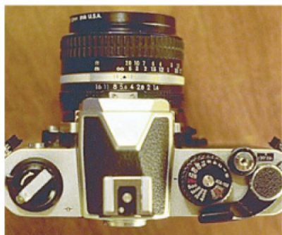
FIGURE 25–4 On this camera, the f -stops and the focusing ring are on the camera lens. Shutter speeds are selected on the small wheel on top of the camera body.
