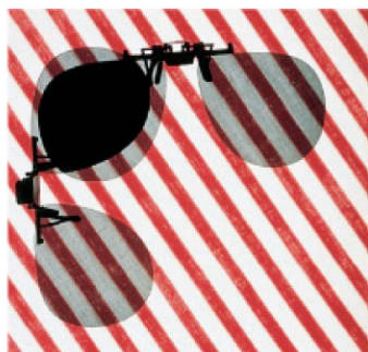
FIGURE 24-44 Crossed Polaroids. When the two polarized sunglass lenses overlap, with axes perpendicular, almost no light passes through.
