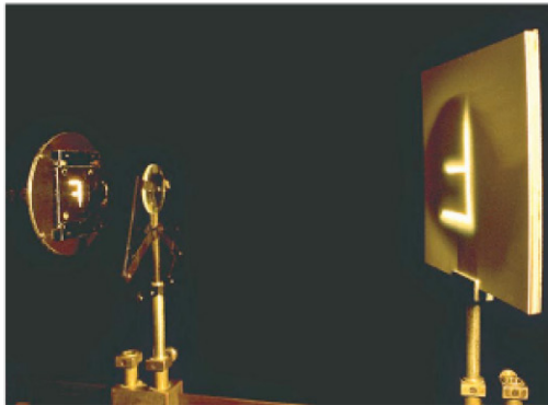
FIGURE 23–30 Converging lens (in holder) forms an image (large “F” on screen at right) of a bright object (illuminated “F” at the left).
