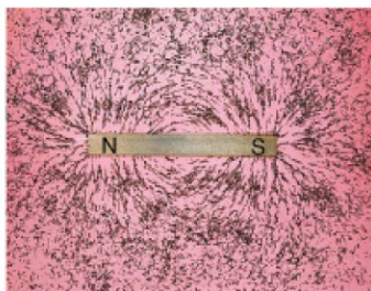
FIGURE 20-41 Iron filings line up along magnetic field lines due to a permanent magnet.
