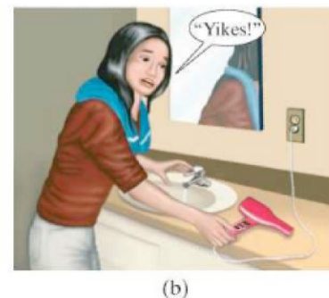
FIGURE 19–25 A person receives an electric shock when the circuit is completed.
