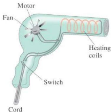
**FIGURE 18–23** A hair dryer. Most of the current goes through the heating coils, a pure resistance; a small part goes to the motor to turn the fan. Example 18–12.
