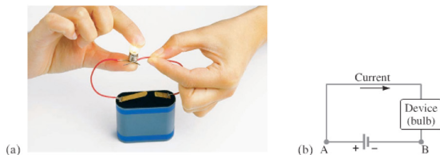
FIGURE 18–6 (a) A simple electric circuit. (b) Schematic drawing of the same circuit, consisting of a battery, connecting wires (thick gray lines), and a lightbulb or other device.
