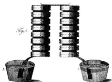
FIGURE 18–2 A voltaic battery, from Volta’s original publication.
