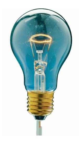
The glow of the thin wire filament of a lightbulb is caused by the electric current passing through it. Electric energy is transformed to thermal energy (via collisions between moving electrons and atoms of the wire), which causes the wire's temperature to become so high that it glows. Electric current and electric power in electric circuits are of basic importance in everyday life. We examine both dc and ac in this Chapter, and include the microscopic analysis of electric current.
