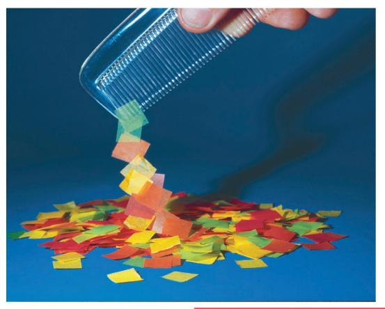
This comb has acquired a static electric charge, either from passing through hair, or being rubbed by a cloth or paper towel. The electrical charge on the comb induces a polarization (separation of charge) in scraps of paper, and thus attracts them.
