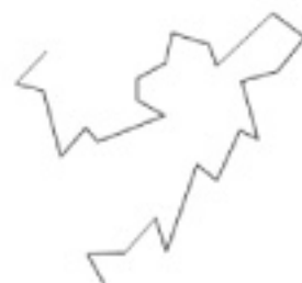
FIGURE 13–1 Path of a tiny particle (pollen grain, for example) suspended in water. The straight lines connect observed positions of the particle at equal time intervals.
