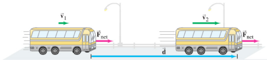
FIGURE 6-7 A constant net force F_{\text{net}} accelerates a bus from speed v_1 to speed v_2 over a displacement d . The net work done is W_{\text{net}} = F_{\text{net}}d .
