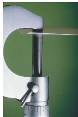
FIGURE 1-11 Example 1-7. A micrometer, which is used for measuring small thicknesses.
