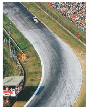
FIGURE 5–12 Race car heading into a curve. From the tire marks we see that most cars experienced a sufficient friction force to give them the needed centripetal acceleration for rounding the curve safely. But, we also see tire tracks of cars on which there was not sufficient force—and which followed more nearly straight-line paths.
